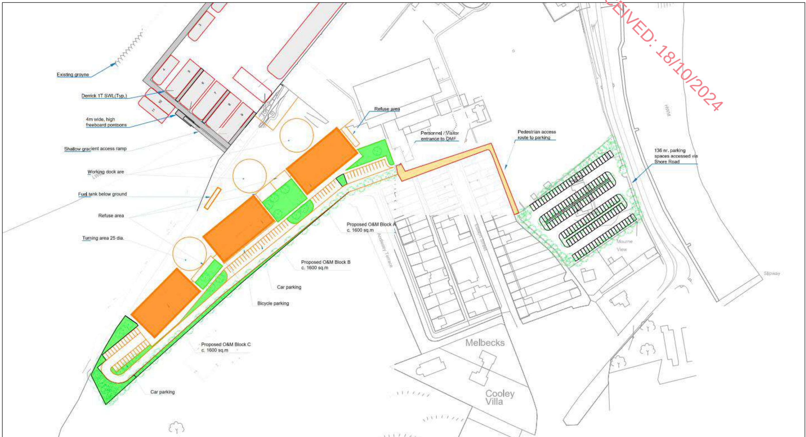
Figure 3-1 General Arrangement plan for proposed developments (extract from the drawing ref.P22034_D4210_D01_proposed facility general arrangement)
